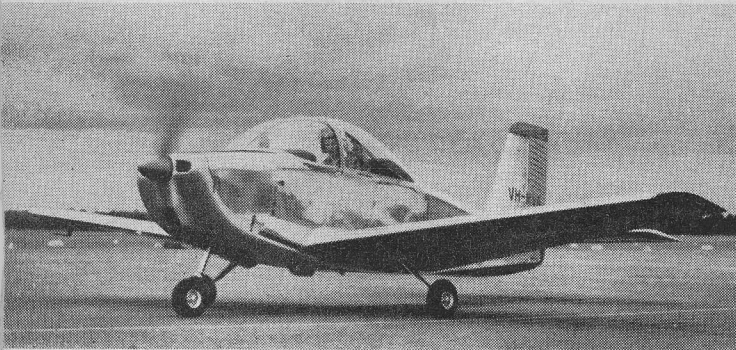
First flight and ground views of the Victa Air Tourer Mk. 11, VH-MVA, taken at Bankstown on December 12. Test pilot Randy Green reported that "everything went entirely as planned for the half hour the Air Tourer was up. The aircraft handled delightfully, cruising comfortably at 106 knots (at 2600 rpm, ht. 1500 ft.)." Tests are proceeding.
