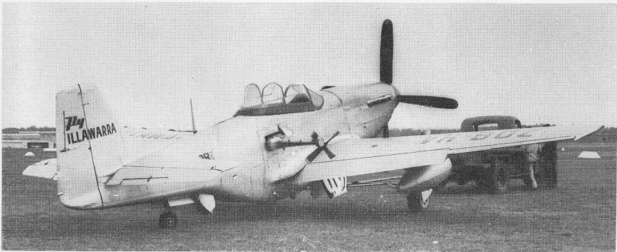
The winch gear and modified canopy (to allow for seating of winch operator) on an Illawarra Mustang aircraft used for Army drogue towing operations. A close-up view of these items is shown in the photograph below of the same aircraft.
