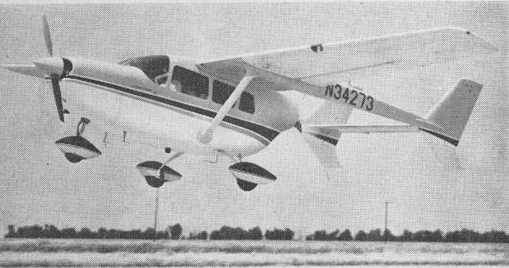
Scheduled for market release next May, Cessna's "push-pull" Skymaster (two 210 hp Continental 10-360 engines) taking off with front engine stopped and propeller feathered.
