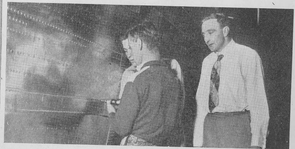
In charge of the airframe overhaul shop is E. Wootton; he is shown supervising a DC-3 mainplane reskinning.
