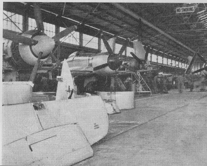
Above: Sea Fury and Firefly aircraft under a work survey before transfer to the repair line. Below: Sea Fury aircraft under repair and modification. Left: Firefly Mk.5 aircraft under conversion for the RAN to Mk.6 standard.
