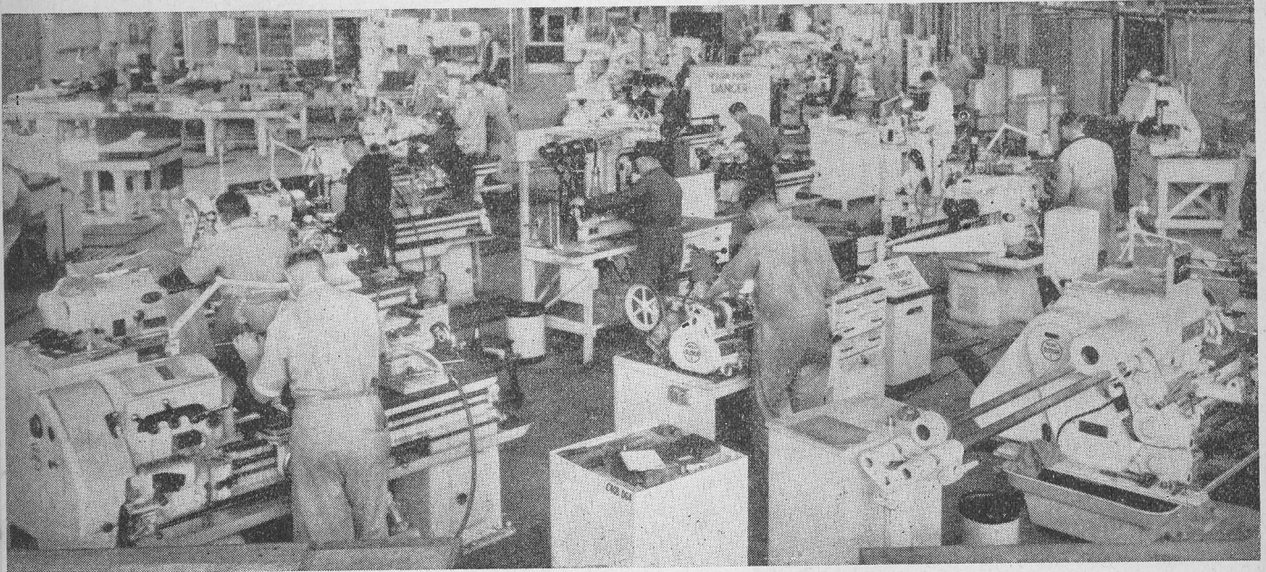
The combined machine shop and toolroom. In the foreground can be seen a small portion of the wood tooling section, which is engaged in the production of economic tools and templates.
