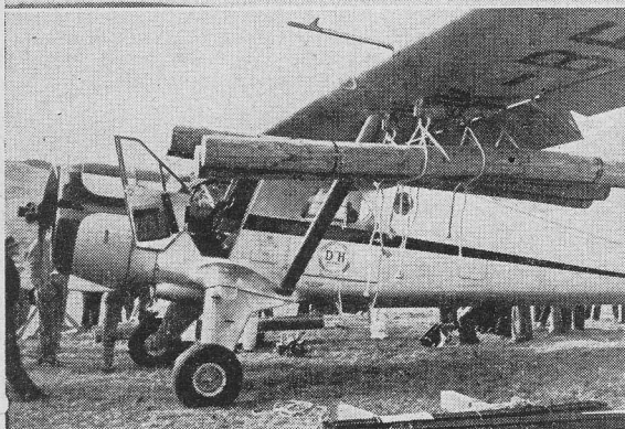
THE BEAVER SHOWING WING ATTACHMENTS Posts being carried on supply-dropping racks of the De Havilland Beaver. The posts are 11 ft. long and 8 in. in diameter and weigh approximately 130 lb. each.
